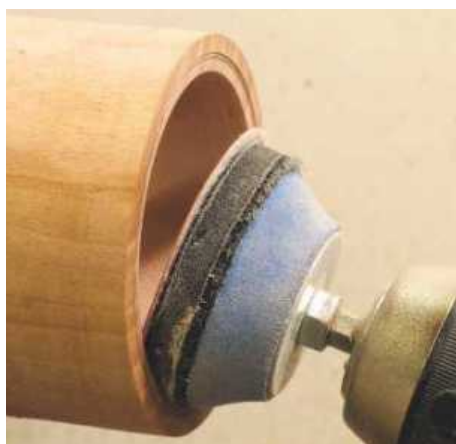
STEP 17. A power sanding pad used inside the vessel is the best option here – I use the 50mm Simon Hope sanding pad, which just fits in and will sand more accurately and generate less heat inside the piece. Heat caused by friction can crack the timber and fruitwoods are particularly prone to this
